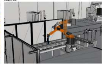
Figure 8: Optimized production process variant 2 and initiated machine-robot control (software: HAL Robotics Framework).
