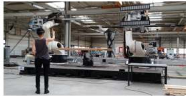
Figure 2. Human wearing an HMD controls the robotic fabrication setup
